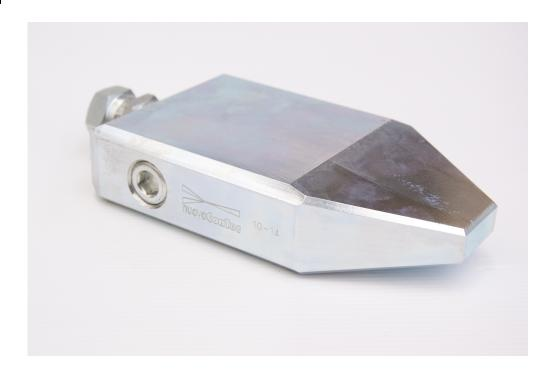
The **Piave** nozzle is used to remove sand. It has a 1/2" F rotating connection and it is fitted with ceramic inserts.
